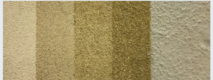
Concrete Primer Basecoat and Silica Sand Broadcast Coat 2nd Basecoat Silica Sand Broadcast Coat Pigmented Topcoat
