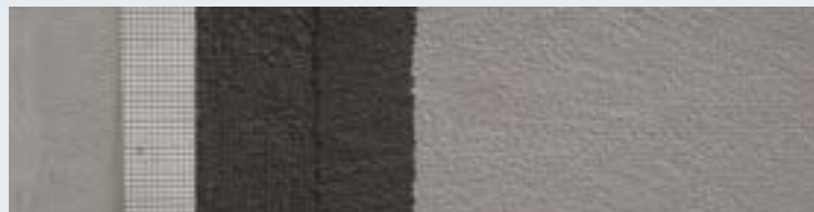
Substrate Fiberlath Base Coat Slurry Coat Pigmented Acrylic Topcoat
