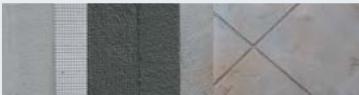
Substrate Fiberlath Base Coat Slurry Coat Grout Coat Texture Coat, Stain and Sealer
