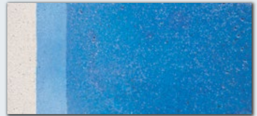
Grind Stain Protective Seal
